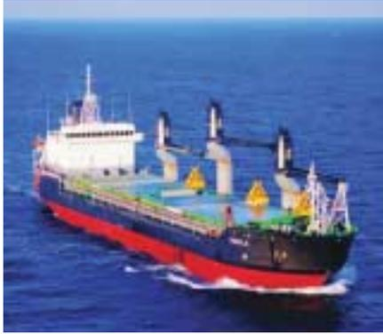
Today, most maritime cranes are operated by remote controls. This ship fitted with Mac Gregor cranes can be tandem operated increasing the maximum load that can be carried.
