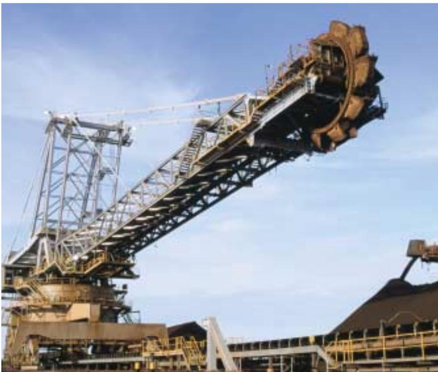
*This 18000 tonnes heavy machine is operated by a Cavotec Micro-control RRC. The most reliable and modern technology is used to ensure smooth operation, as an operational stop is to be avoided at all costs.*
